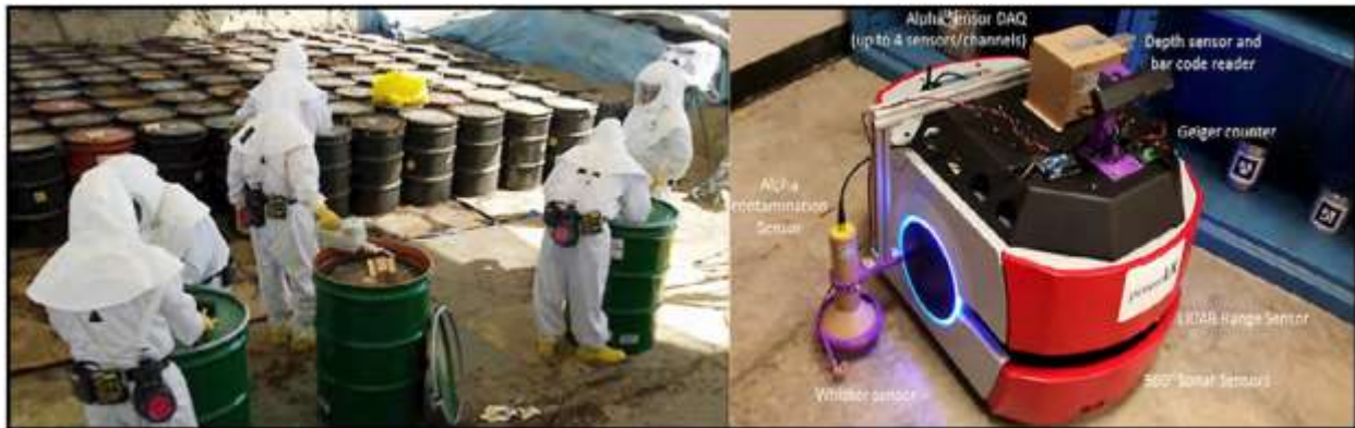
Fig. 4. (Left) Inspection of low-level waste at WIPP storage facility.[3] (Right) A mobile robot platform developed at UT Austin and LANL to perform inventory, radiation survey, and detection of alpha contamination in storage facilities for SNM. Source: UT Austin NRG.
