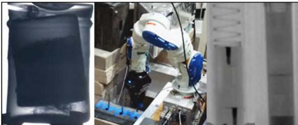
Fig. 8. (Left) Radiograph of non-3013-packaged solids with a container breach. (Center) Industrial manipulator used to produce neutron radiography images in both a reactor beam port and using a portable neutron source. (Right) Image of spent nuclear fuel rod with robotic system with gadolinium and tungsten inclusions.[8]
