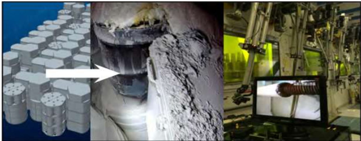
Fig. 3. (Left and Center) Drum explosion accident at WIPP. Robots were needed to assess damage, determine root cause, and act to contain any further spread. (Right) Hot cell master/slave manipulators for routine radioactive material handling [3] could be replaced by off-the-shelf industrial robots enabled by 3D sensing and smart software. Source: DOE-EM Presentation to UT Austin Nuclear and Applied Robotics Group (NRG).
