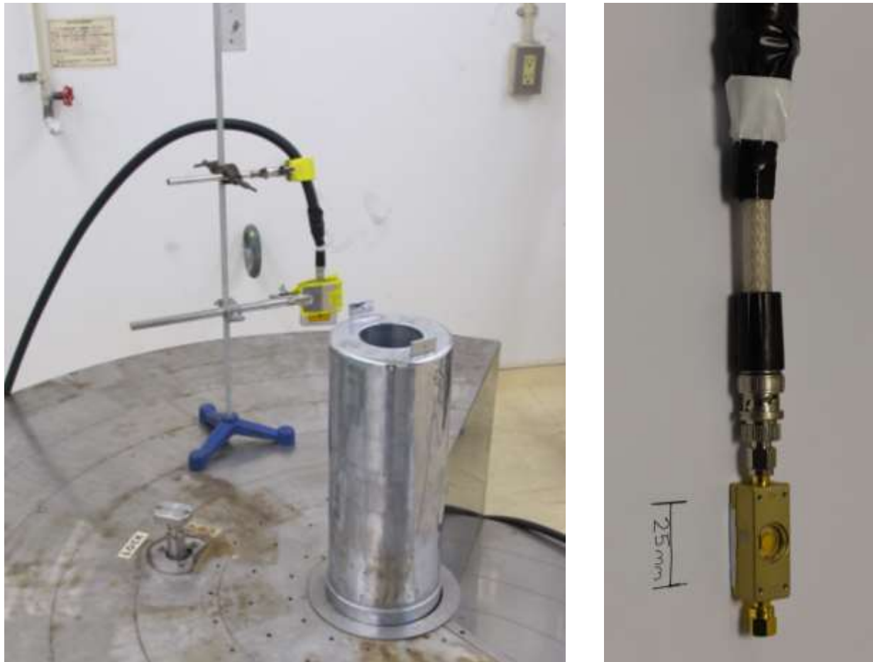
Figure 2. (Left) diamond detector C1 in Co-60 irradiation facility and (right) diamond detector S1 located at the end of a 50 m cable run.
