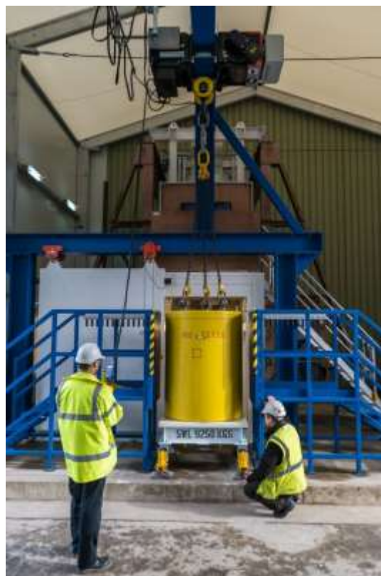
FIGURE 7: DCIC Hoist, Import/Export Facility Structural Steelwork and Bogie Transfer System
