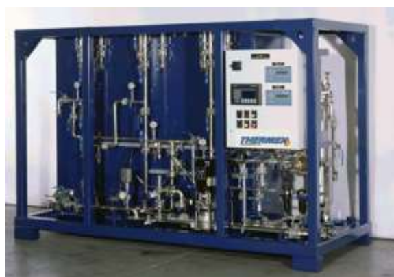
Figure 2 — Typical EnergySolutions' mobile demineralization system.
