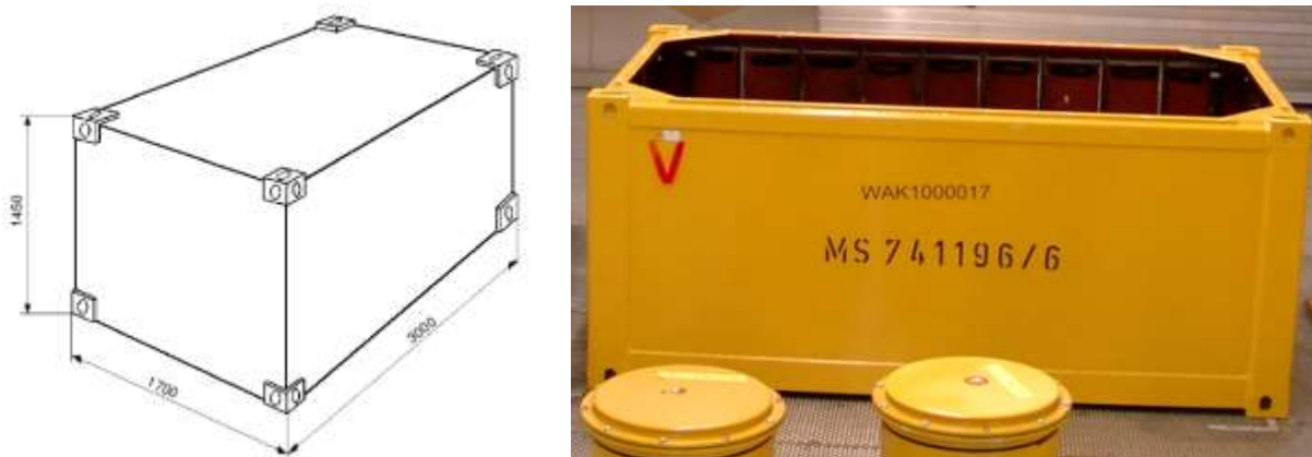
Figure 3: Technical specification and photograph of Konrad Type 4 Container (the dimensions in the drawing are in millimeters)
