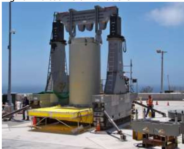
Fig. 6. Holtec Below Grade CTF
