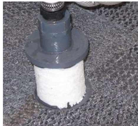
Fig. 6. Examples of Dewatering Verification Filters, Placed into Unused Condensate Filter Demineralizer Liners
