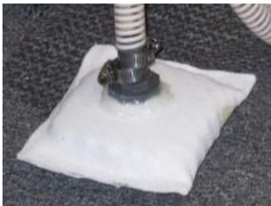
Fig. 6. Examples of Dewatering Verification Filters, Placed into Unused Condensate Filter Demineralizer Liners
