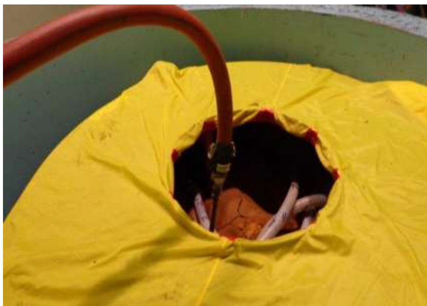
Fig. 5. Dewatering Verification Filter, inserted into a filled and dried CFD resin liner.
