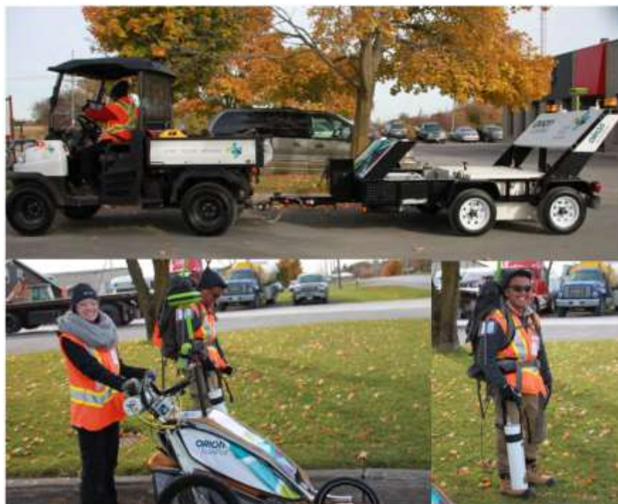
Figure 3: Examples of ScanPlot SM Platforms used for the Gamma Surveys
