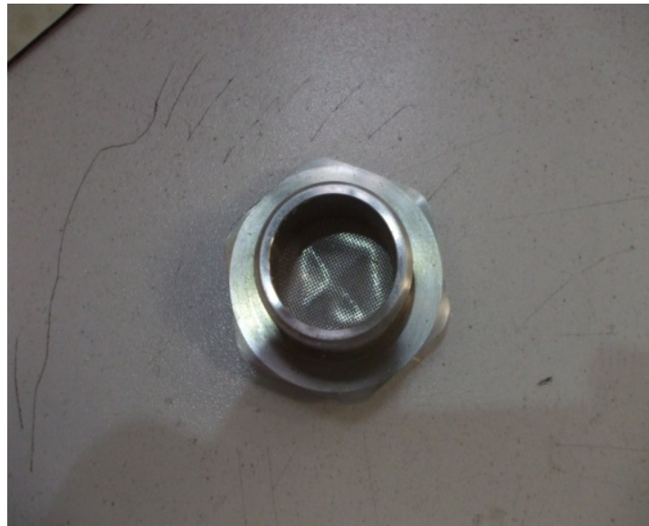
Figure 9 – Filter deformation post 20 bar burst test
