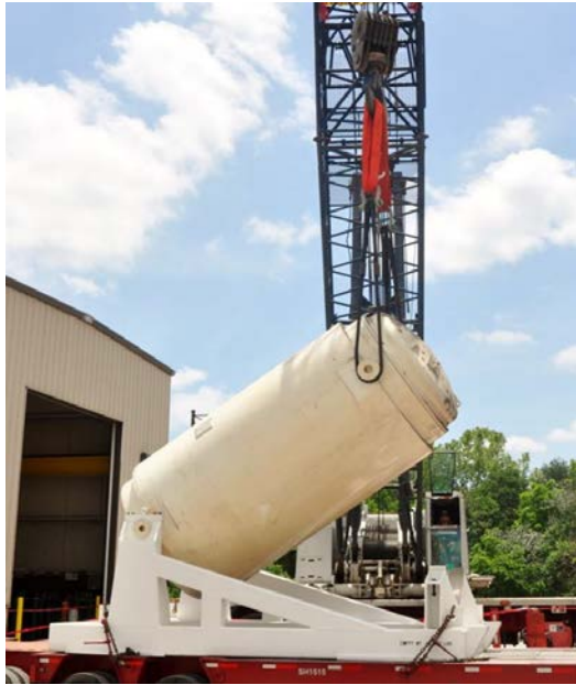
Fig. 2. TN-32B Cask at Fabricator
