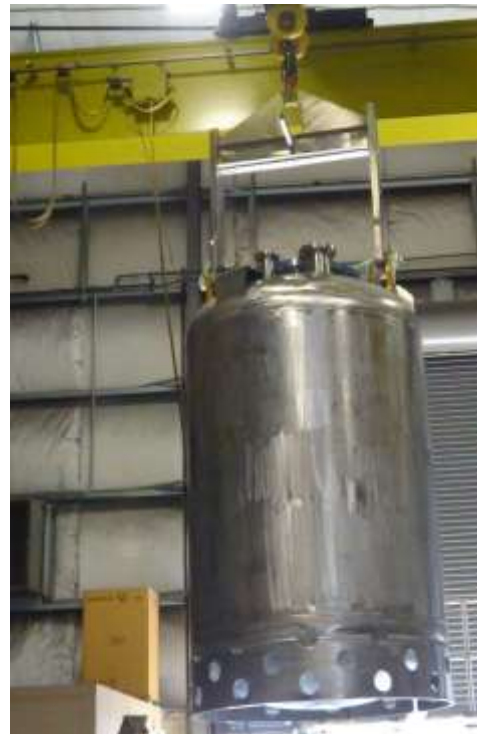
Fig. 10: Completed Fabrication of First STSC
