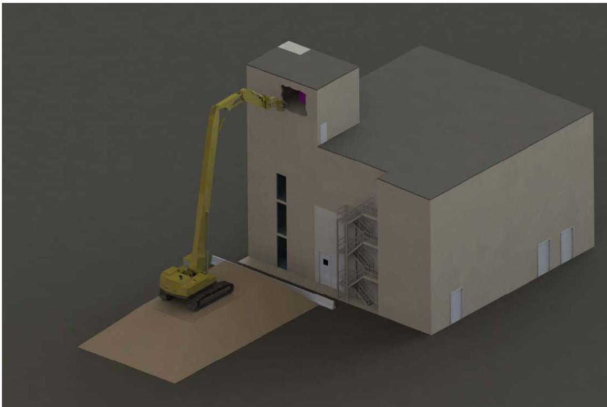
Computer model of surgical removal of column glove box on the 6 th floor of PRF.
