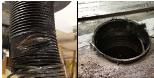
Figure 2: Damaged closure bolt (left) and deformed bolt hole (right) on a 8-120B cask
