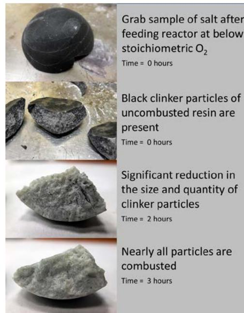
Figure 2: Qualitative experimental results from non-stoichiometric oxidation experiments and subsequent oxidation. Carbon clinker in the melt was observed to oxidize fully after 3 hours.
