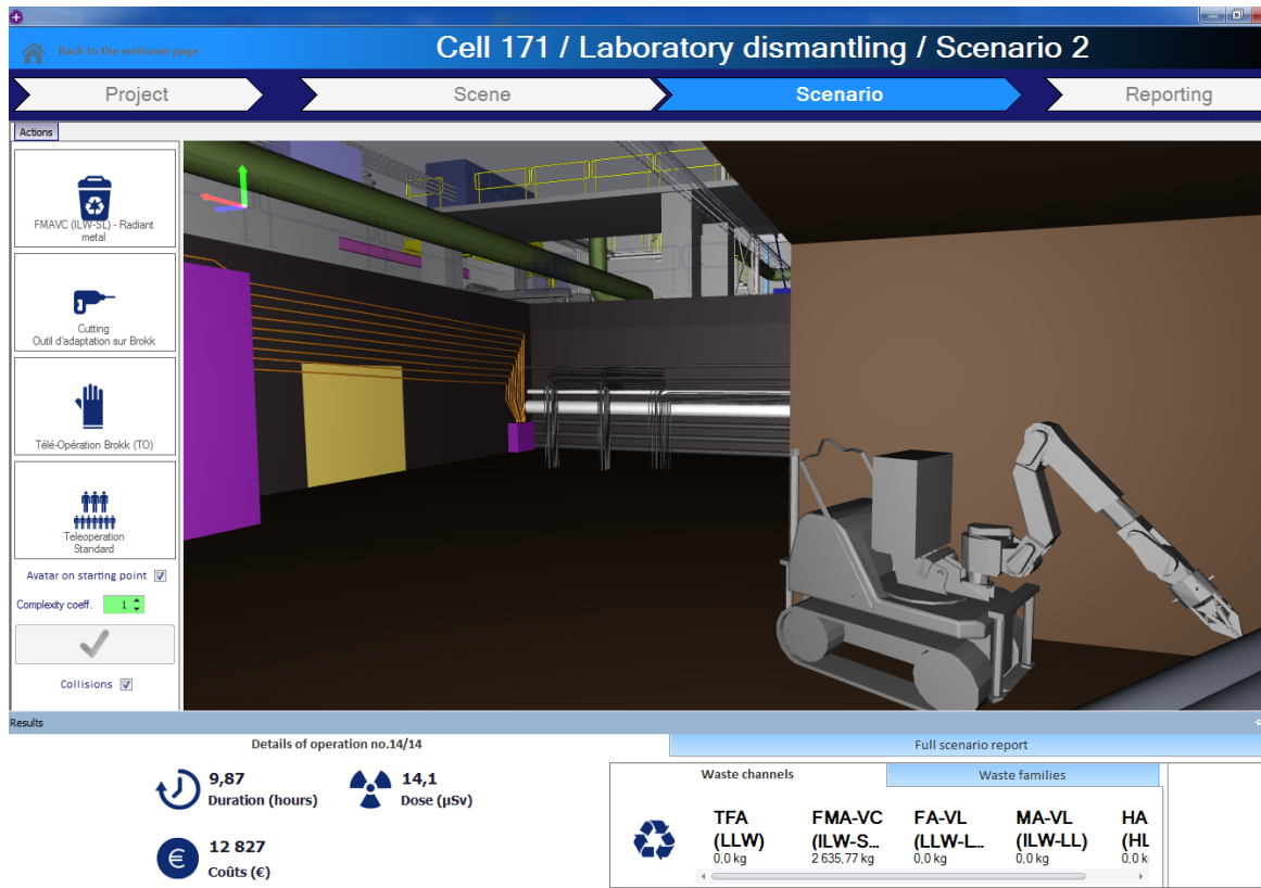
Fig 1. Simulating an operation on DEMplus® is done by selecting the equipment, choosing the type of operation to be simulated and the tool and team to be used. The results are provided in term of cost, dose, duration, and waste generated.
