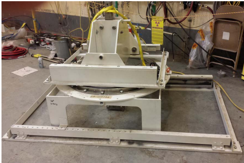
Figure 8. The tool deployer offered full rotational capability for tools to reach piping that was offset from the hatch opening.
