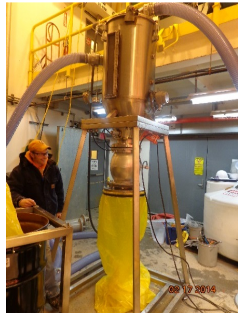
Figure 3. Mockup testing of HEPA filtered vacuum system for Raschig ring removal.
