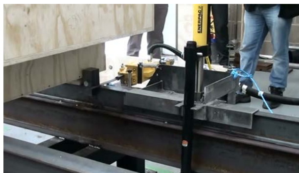
Fig. 4. Wheel Block Removal Tool Trial
