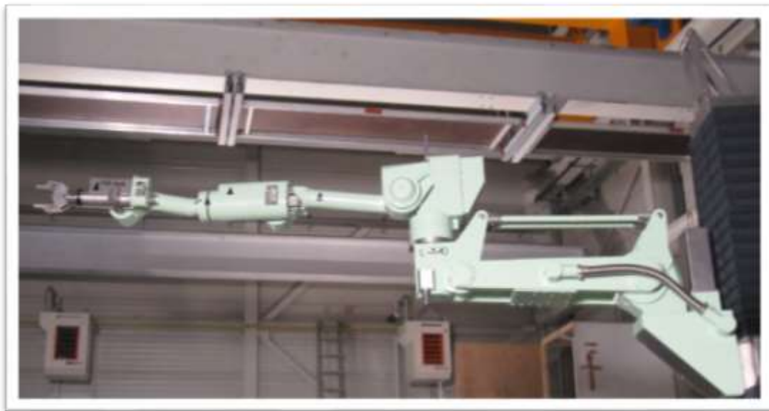
Fig. 1. Maximum Horizontal Reach: 4 m (13 ft)
