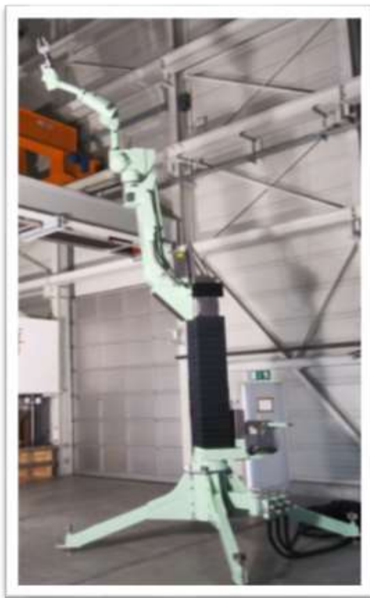
Fig. 2. Max. vertical reach of 7 m (23 ft) Fig. 3. Dimensions of PPS and A1000S
