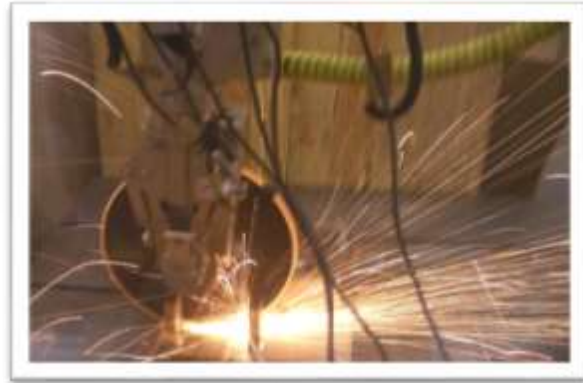
Fig. 6. X: cutting direction, Z: cutting depth Fig. 7. Cutting with angle grinder
