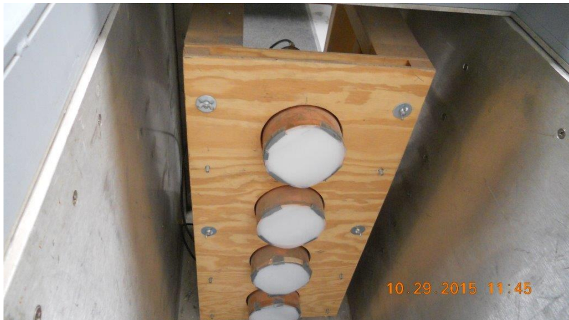
Fig. 2. Phoswich detectors in the ZEUS system
