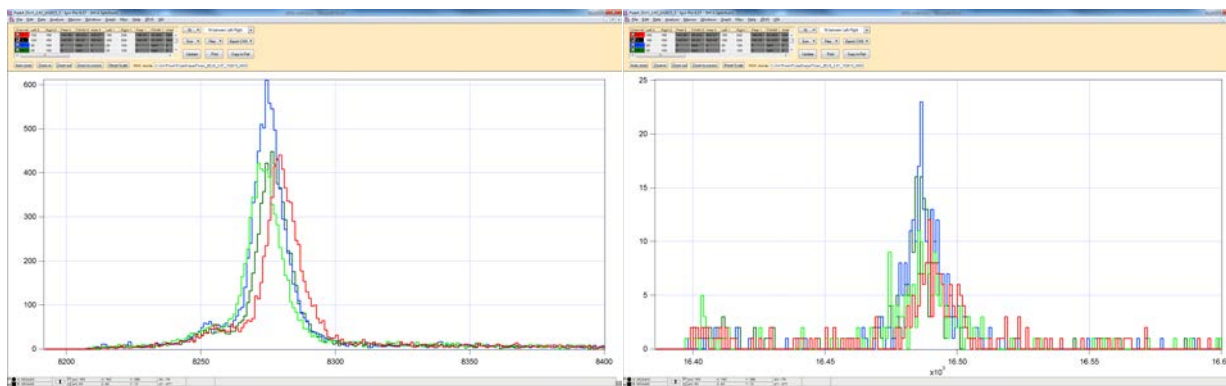
Fig. 9 CsI and “in-between” spectra for the four ZEUS detectors (energy range \approx 0-200keV displayed)
