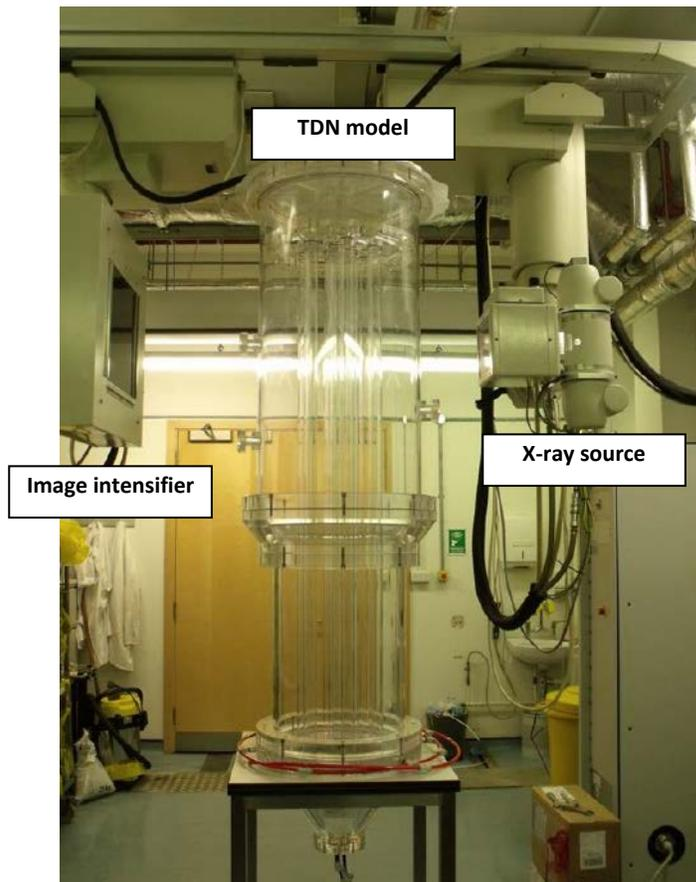
Figure 5: Perspex Model in the X-ray Cell at UCL [8]
