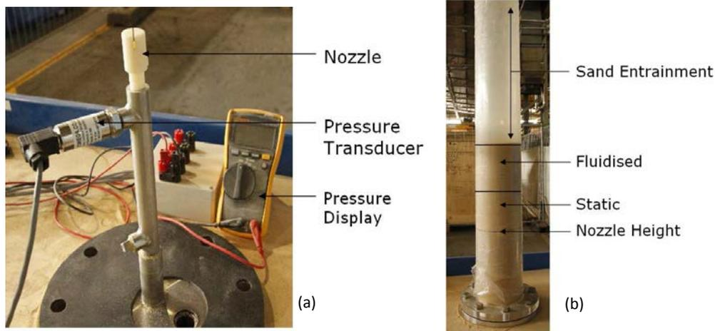
Figure 3: NNL rig arrangements [4, 5], (a) Pressure measurements, (b) Perspex column for fluidisation quality analysis
