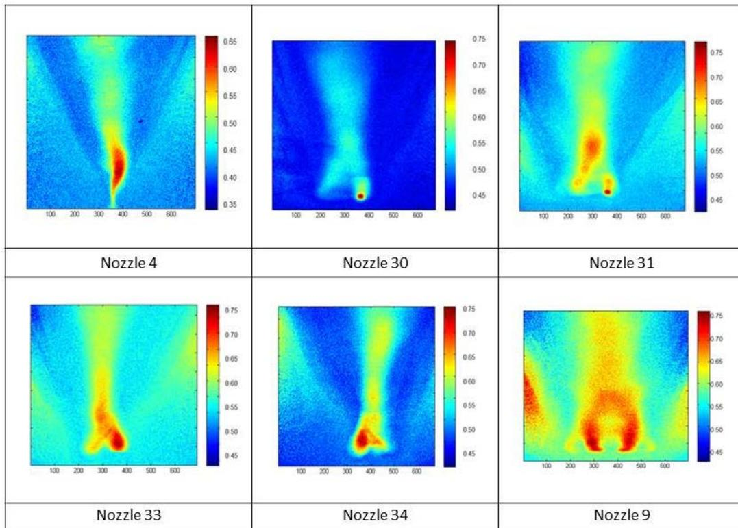
Figure 8: Average voidage profiles for peripheral nozzles in sand (720 images per nozzle) [10]
