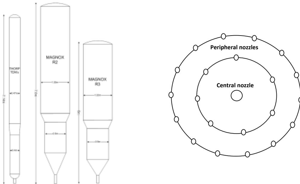
Figure 1: General schematic of Sellafeld Ltd TDN reactors (left) [2], section of conical base (right).
