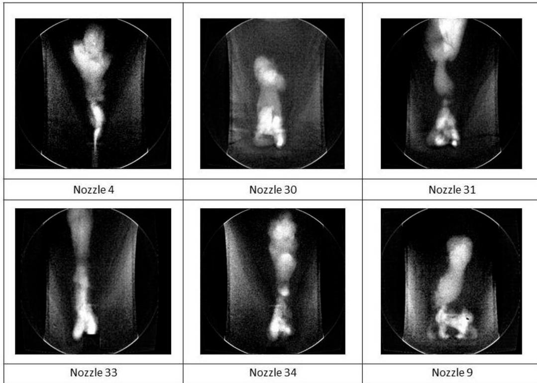
Figure 7: X-ray Images of jet penetration in sand at a 90 litres per minute flow rate [10]
