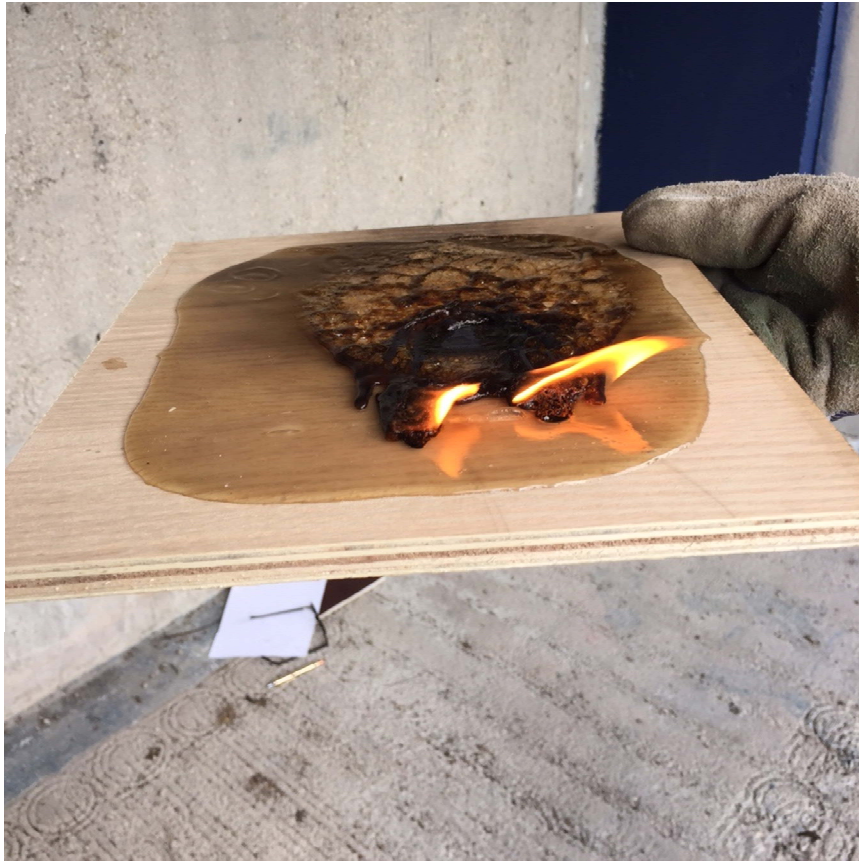
Figure 6. Fixative continuing to burn after exposure to direct flame.
