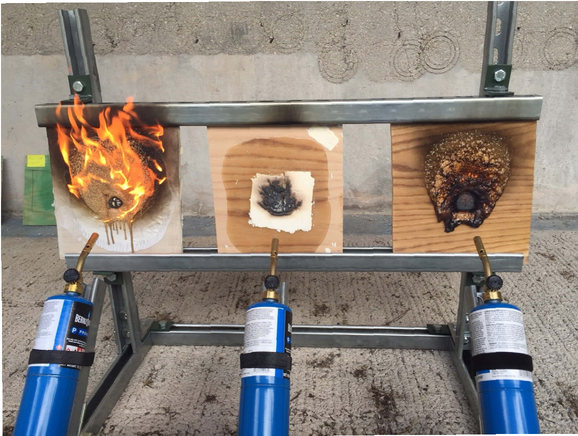
Figure 5. Fixative and intumescent coating coupons reacting to direct flame source.
