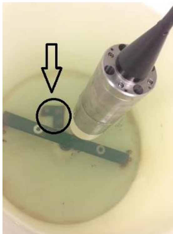
Fig. 4. Setup to test the ability of the 3-D sonar to image a 6-mm thick metal piece.
