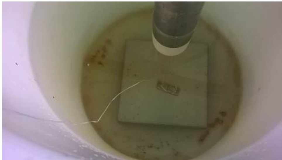
Fig. 12. Test setup in small tank with 3D sonar and small stacked metal plates
