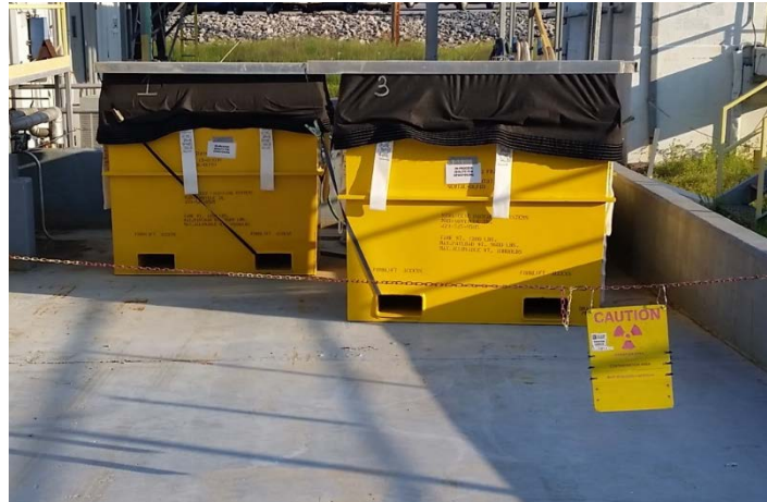
Figure 2 – Zeolite in dewatering bags in frames
