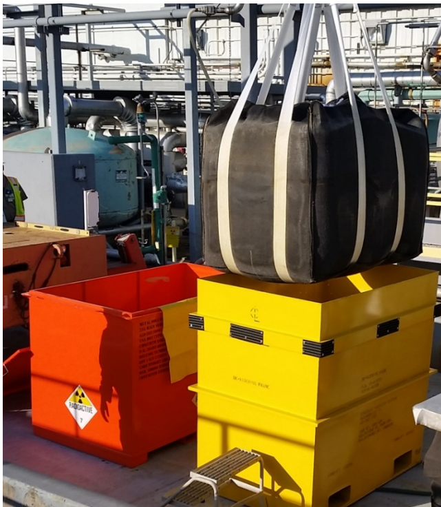
Figure 4 – Dewatering bag lifted out of the frame
