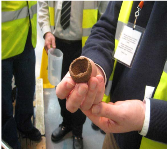
Figure 5. Sludge sample collected using freeze sampling probe. [3]
