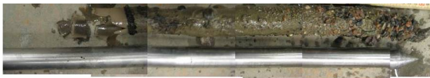
Figure 6. Reverse freeze core sample collected using freeze technology. [3]
