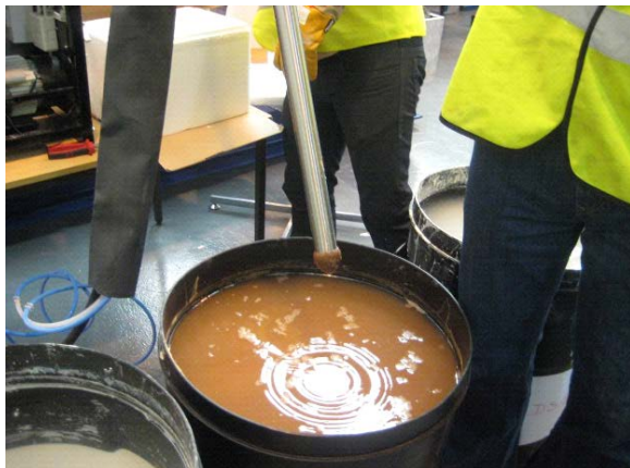
Figure 4. Freeze sample being collected from simulated sludge. [3]
