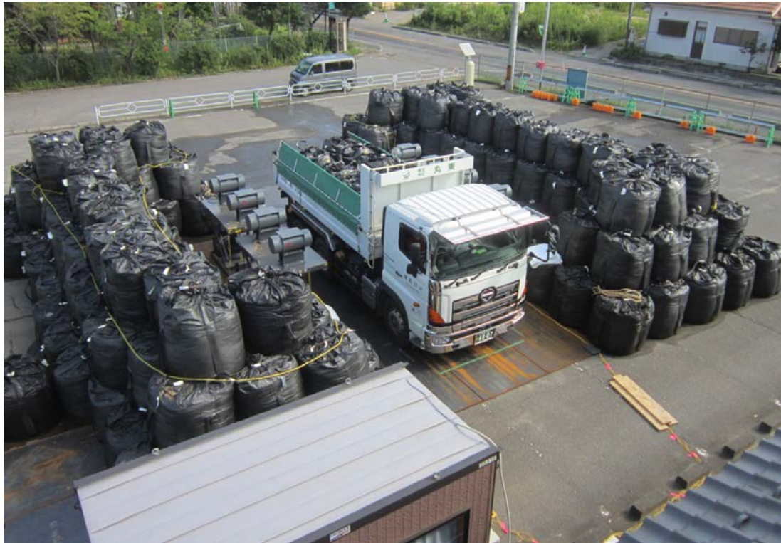
Figure 2 TruckScan during Fukushima testing. The shield wall here is built from sacks filled with clean soil.
