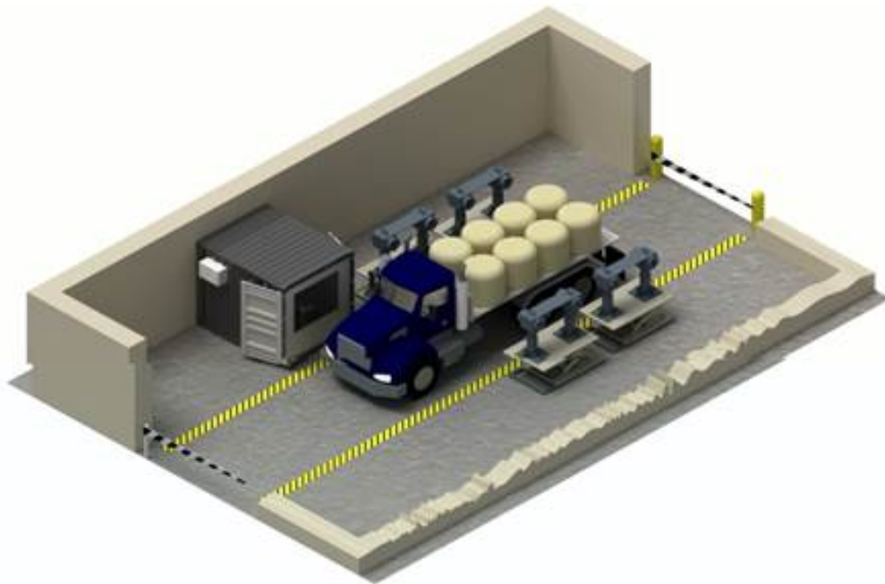
Figure 1 Graphical illustration of TruckScan system at site. Concrete shield wall shown here.
