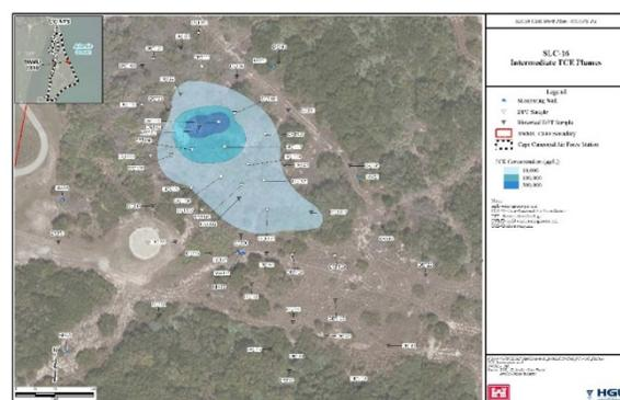
Figure 17 Intermediate Depth TCE Groundwater Results
