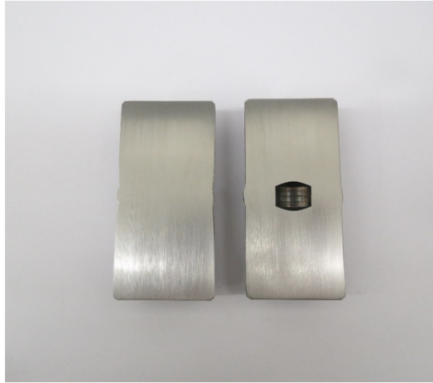
Figure 3. Artificial pore before HIP (right) and after HIP (left).
