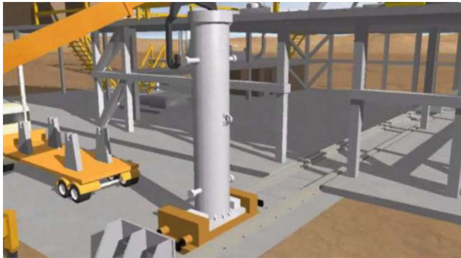
Fig. 4. Visualization of the transfer cask set on the transfer carrier, for locating waste packages directly over the borehole and under the drill rig.
