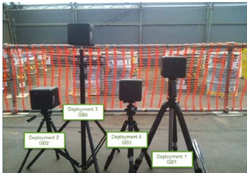
Figure 2 - Deployment of four GrayQb™ devices facing area of interest
