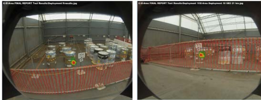
Figure 21 - Test 9 and 10 results demonstrating usefulness of multiple views to triangulate source position in 3D area.
