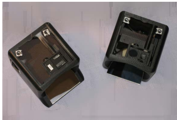
Figure 18 - GrayQb SF2 with internal steel shot shielding (left) and w/o shielding (right)
