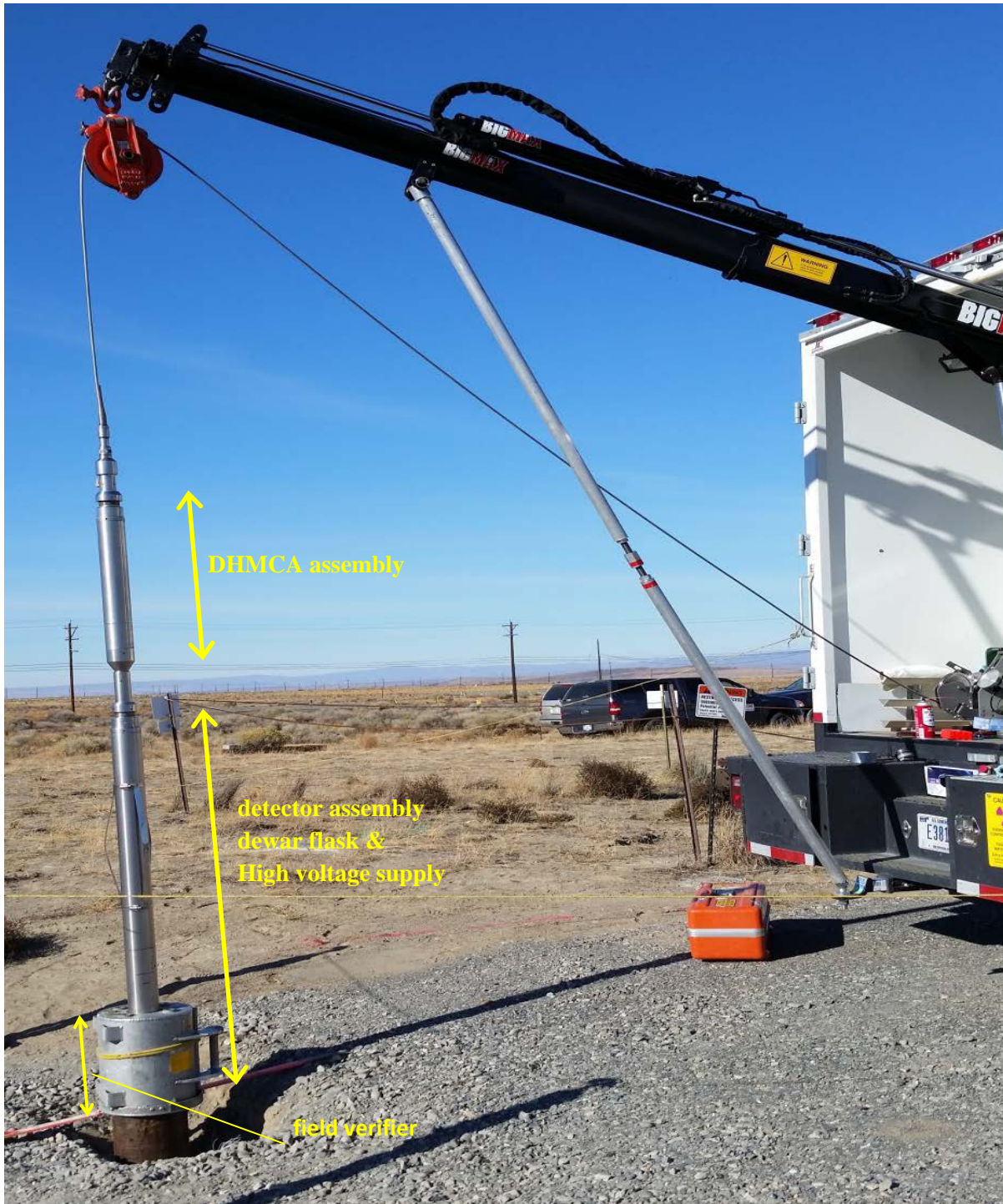
Figure 2. This image shows the 3.375-inch OD DHMCA attached to an SGLS borehole probe collecting a verification measurement in a KUTH verifier.
