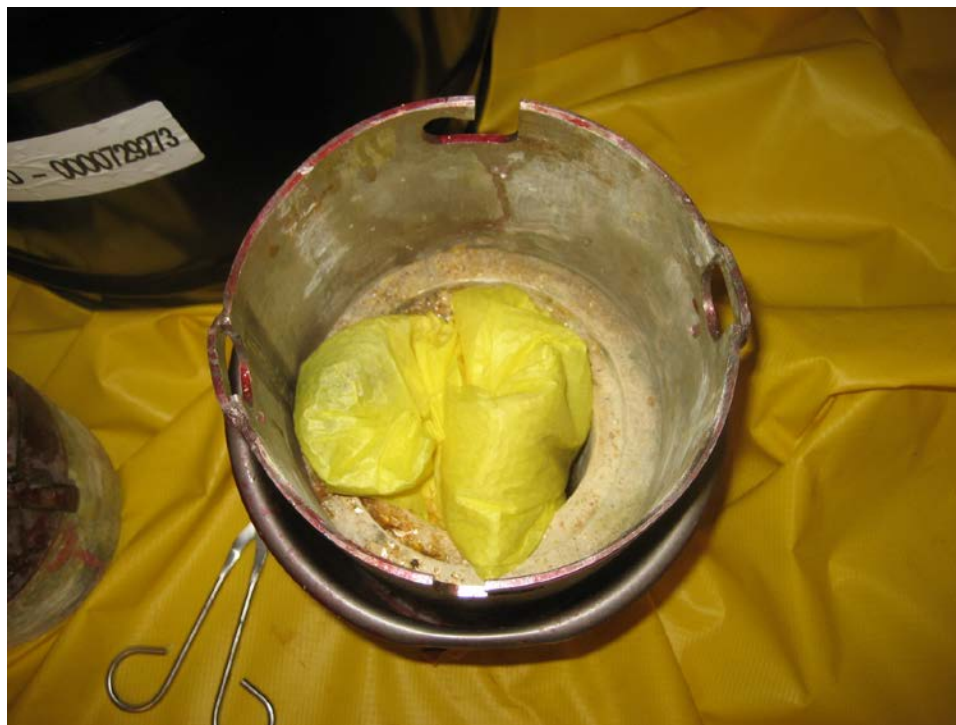
Figure 7: Shielded pig containing wrapped ^{85}\text{Kr} samples.
