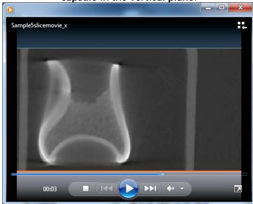
Figure 18: X-ray tomographic image of Capsule 5 cutting across the capsule in the vertical plane.
