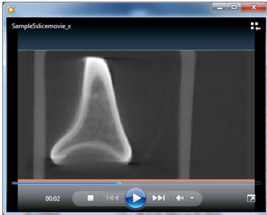
Figure 17: X-ray tomographic image of Capsule 5 cutting across the capsule in the vertical plane.
