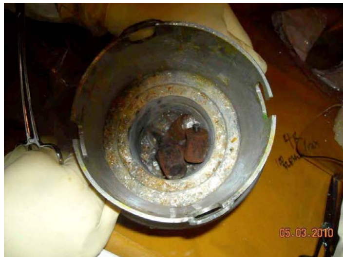
Figure 3: Photo of squashed metal tubes, presumably zeolite 5A HIPed in a glass matrix 6 .
