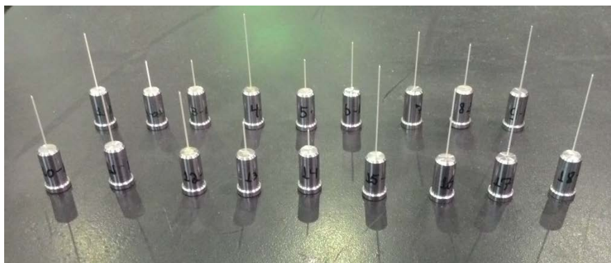
Fig. 1 – Samples in 0.7mm borosilicate capillary.
