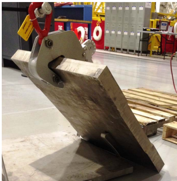
Fig. 7. East Shield Plate Used to Bend Tabs (Mock-up Practice)
