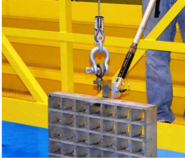
Fig. 6. C-Block Lifting Device on Mock-up Plate in Practice Pool
