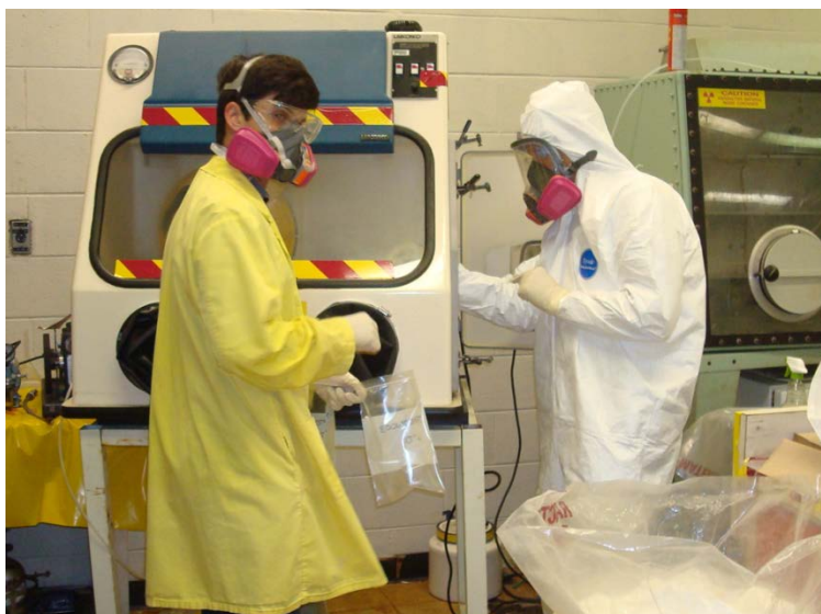
Figure 3. Sub-sampling Contaminated Concrete Cores to Obtain a Defensible Sample for Analysis.
