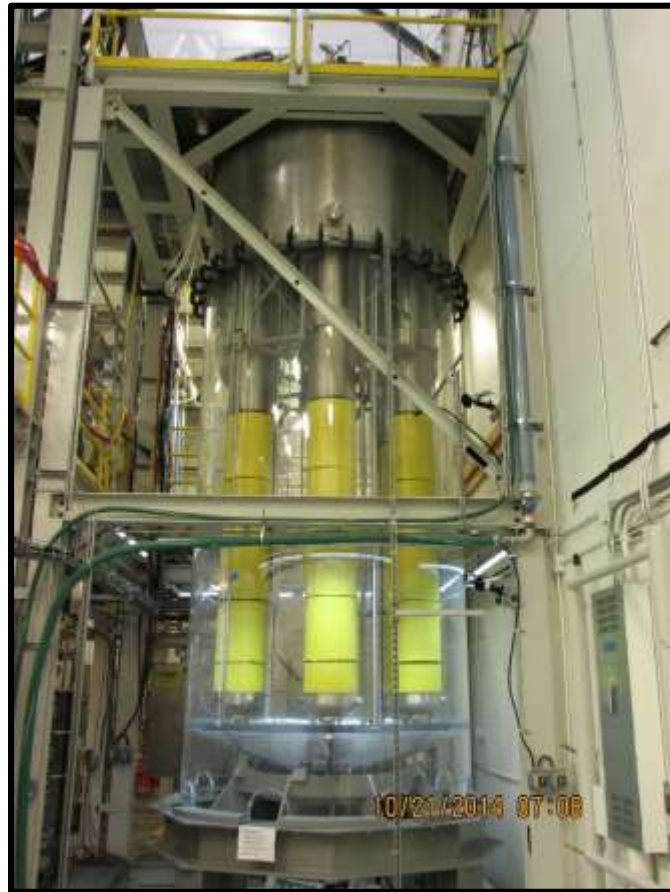
Figure 2. Prototypic (Scaled) PJM Test Vessel
