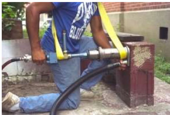
Figure 6. Pentek Rotopeen and Squirrel HEPA vacuumed scabblers being used.
