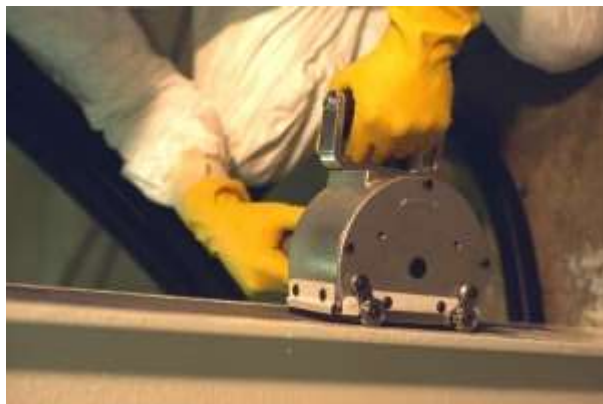
Figure 6. Pentek Rotopeen and Squirrel HEPA vacuumed scabblers being used.
