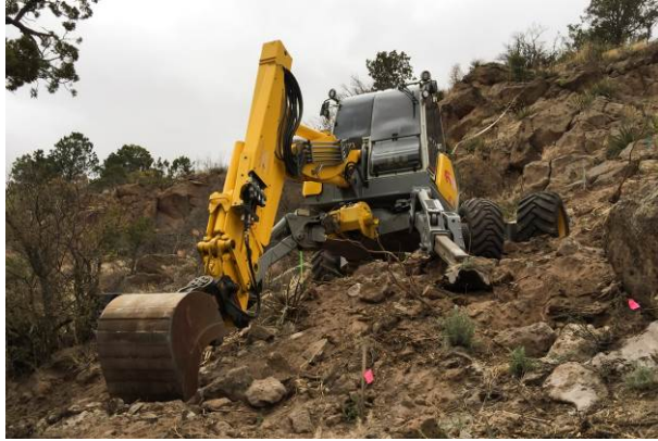
Figure 5. Menzi Muck 91-E spider excavator positioned on the SWMU 32-002(b2) excavation site.
