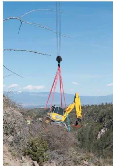
Figure 4. Photos of Linkbelt ATC 3275 lifting and lowering the Menzi Muck Spider Excavator to the excavation site. Photos courtesy of Los Alamos National Laboratory.
