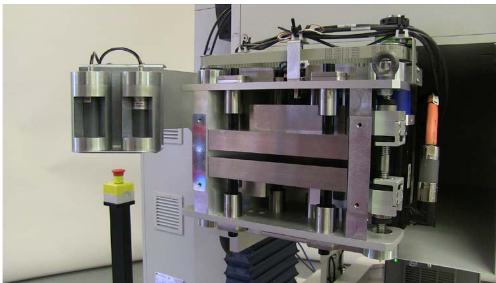
Fig. 4. The Geiger-Muller detectors and the variable aperture collimator (with guards removed) in the partially open position are shown in the photograph.
