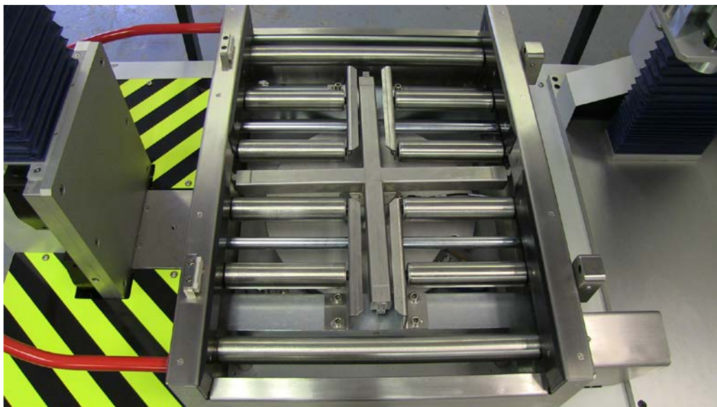
Fig. 3. The cruciform rotator and conveyor rollers are shown in the photograph.
