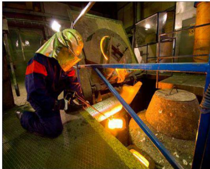
Fig. 1. Induction furnace at Studsvik after completed casting process.
