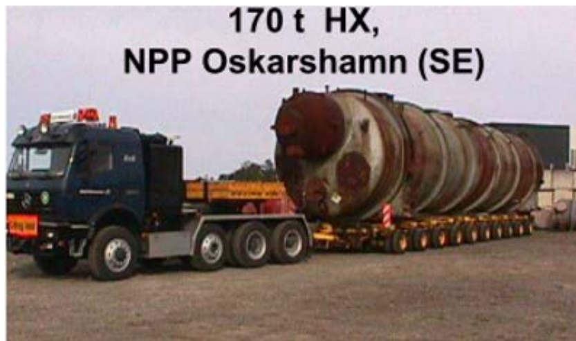
Fig. 3. BWR re-heater during transport to Studsvik for treatment.
