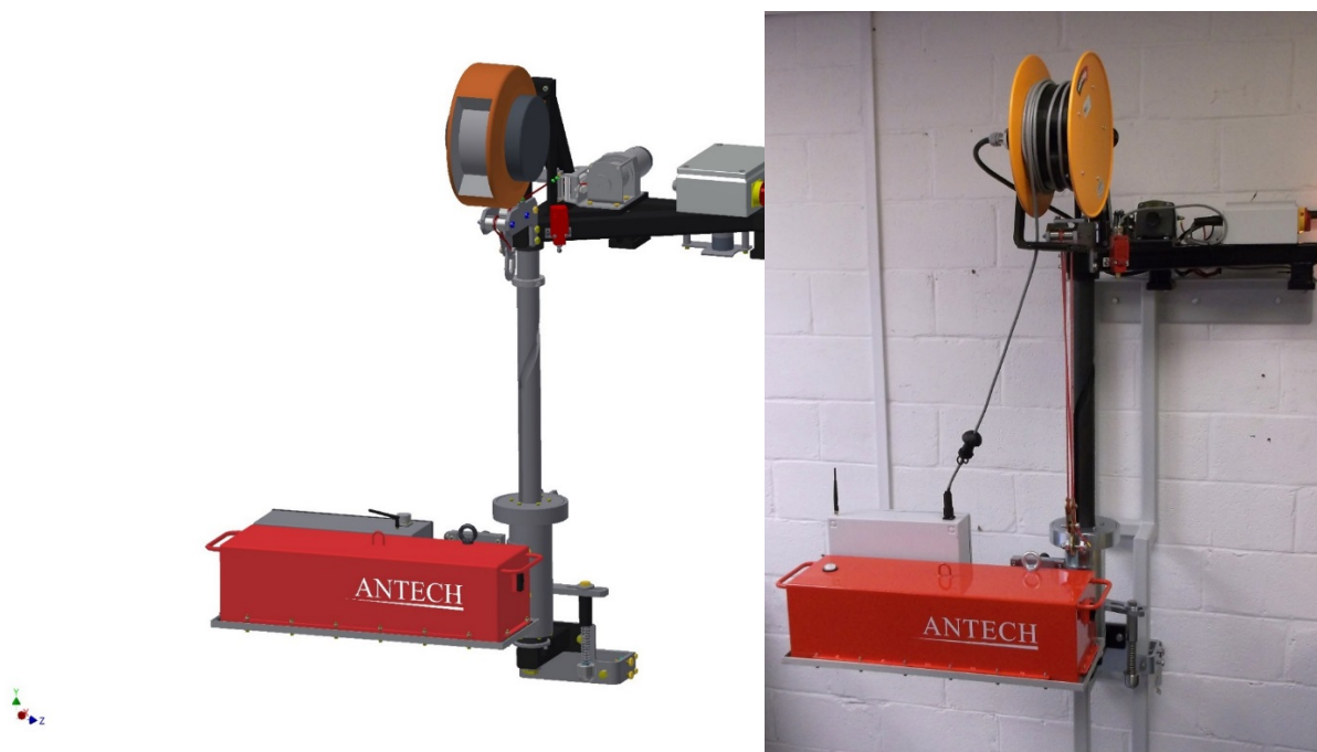
Fig. 4. A design drawing of EMBASSY (left image) is compared to a photograph of EMBASSY mounted in a test rig (right image).
