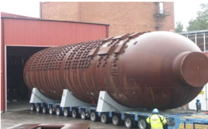
Fig. 3. Magnox Boiler entering Studsvik Melting Facility.
