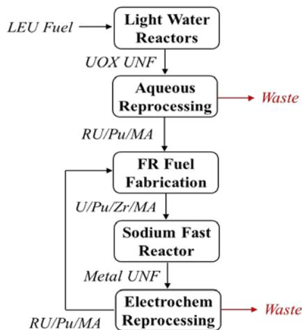
Figure 1. Overall Block Flow Diagram.
