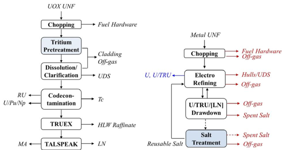
Figure 2. General Aqueous (a) and Electrochemical (b) Separations Process Flowsheets
