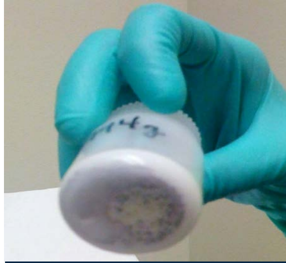
Fig. 1. Technetium dioxide (black precipitant) in groundwater brine simulant
