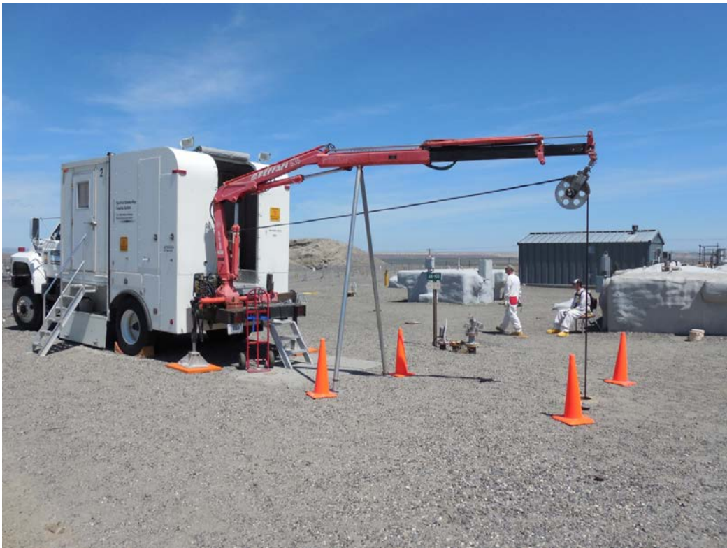
Figure 1. Example setup of logging operations conducted inside tank farm boundary. Logging truck set up on borehole with boom extended towards borehole and borehole probe downhole.
