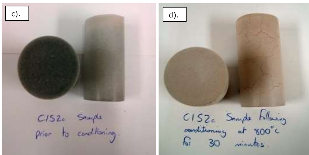
FIGURE X: a). C1S1 at 28 days. b). C1S1 following heating to 800°C. c). C1S2c at 28 days d). C1S2c following heating to 800°C.
