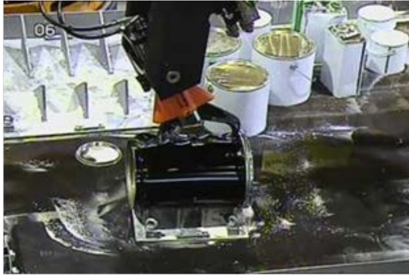
Figure 4: Hydraulic shear being used to disrupt mock-up waste can
