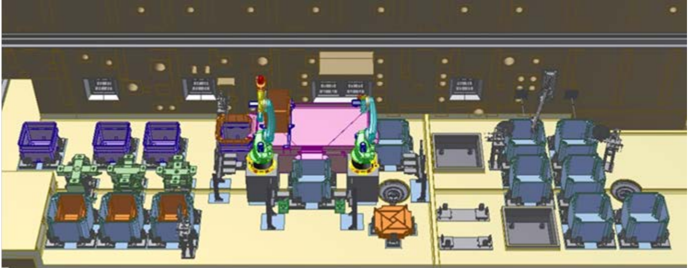
Figure 2: CAD image of proposed layout of the BEP Waste Treatment Cell (WTC)
