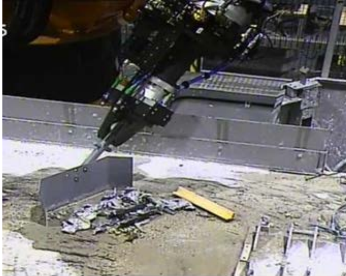
Figure 5: a housekeeping tool for cleaning the table held in the jaw grippers
