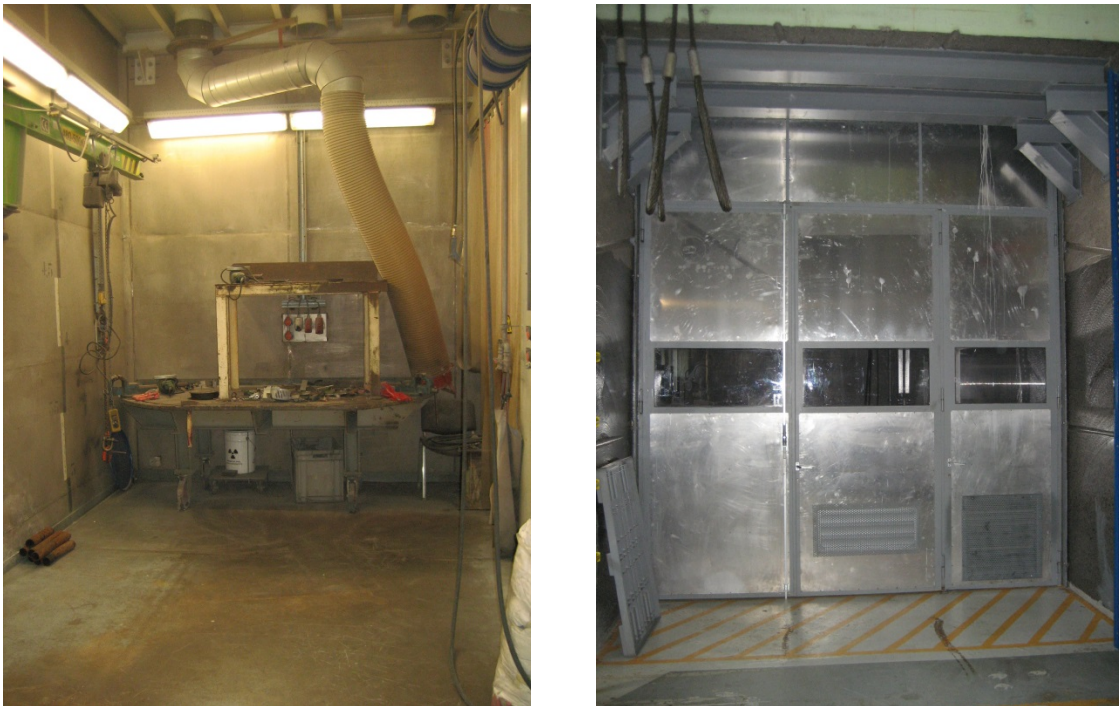
Figure 9: In- and outside view of the cutting and size reduction workshop at BR3
