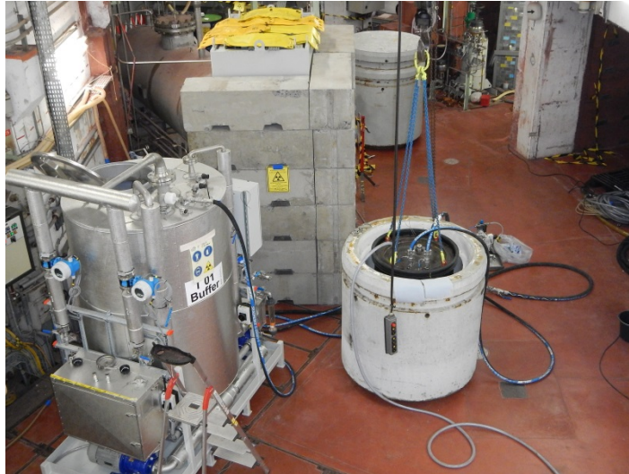
Figure 8: Resin transfer set-up with shielded containers
