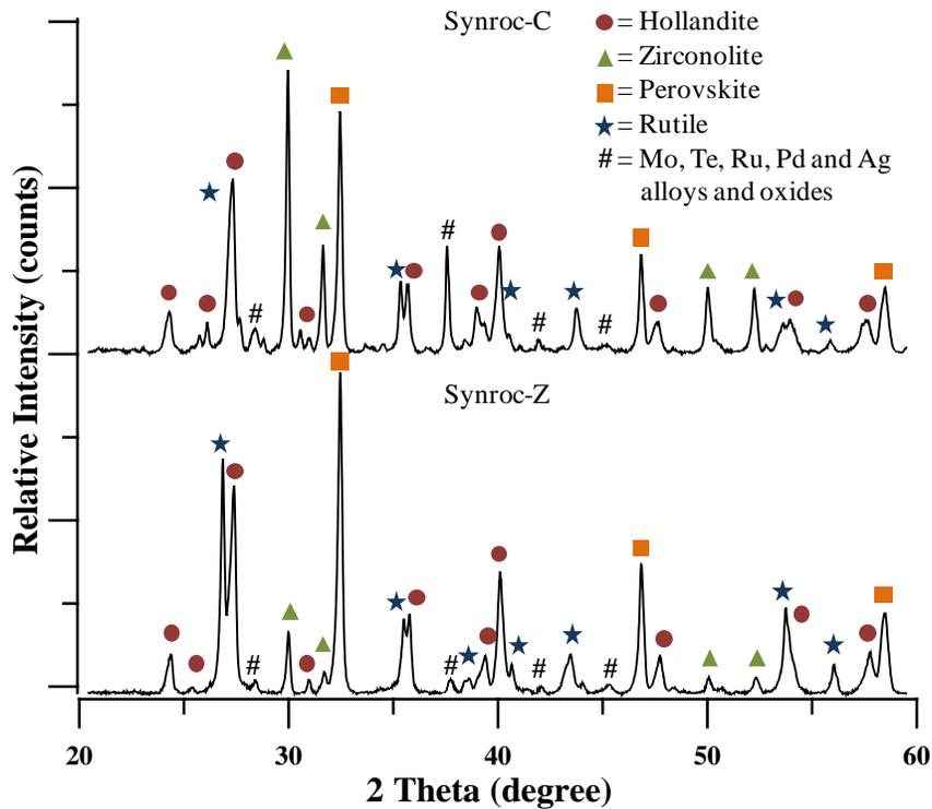
Figure 1. XRD of Synroc samples with 20 wt% simulated HLW, showing a decrease in zirconolite phase in Synroc-Z by a factor of 3-4.
