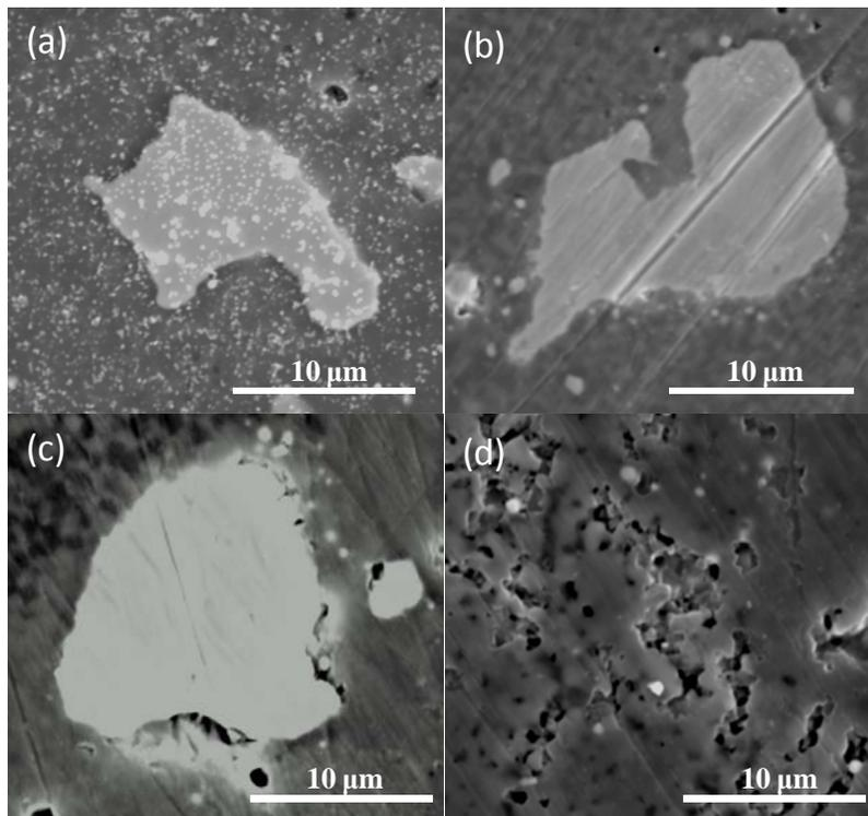
Figure 4. SE images of intermetallic particles (lighter grey) in Synroc-Z with 20 wt% simulated HLW (a) before (polished to 0.25 μm), (b) after 7 days and (c) after 28 days (each ground with 600-grit SiC paper) leach testing and (d) corroded region on Synroc-Z after 28 days leach test particularly in the perovskite-rich region. This indicates that the perovskite is more soluble than other phases.
