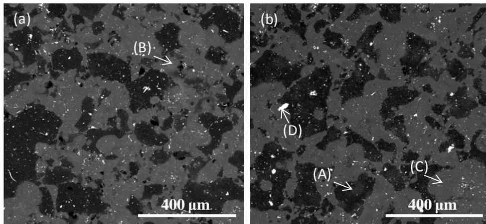
Figure 2. BSE images of (a) Synroc-C and (b) Synroc-Z with 20wt% simulated HLW. Generally, (A) the dark grey phase is rutile, (B) the light grey zirconolite and (C) the intermediate grey a mixture of perovskite and hollandite. (D) White regions are metallic precipitates.
