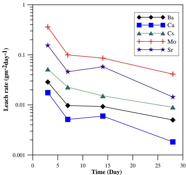
Figure 3. Leach rates of Synroc-Z (20wt% simulated HLW) under static conditions in deionized water at 90°C. The leach rates decreased with leaching time.
