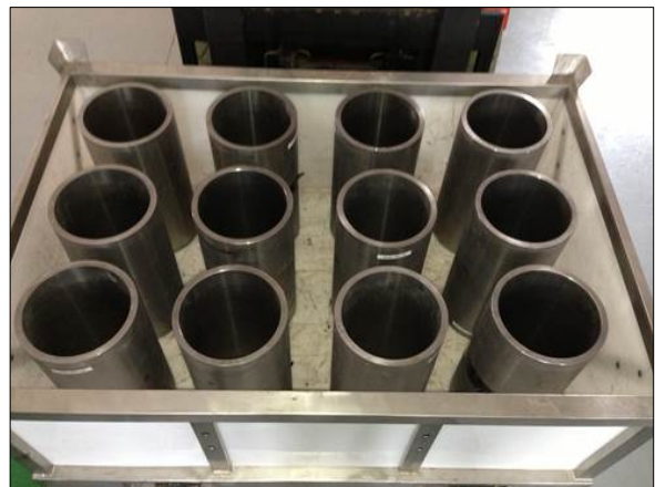
Fig. 19. Metallurgically produced tubes (reference material, Co-60, Ag-110m)
