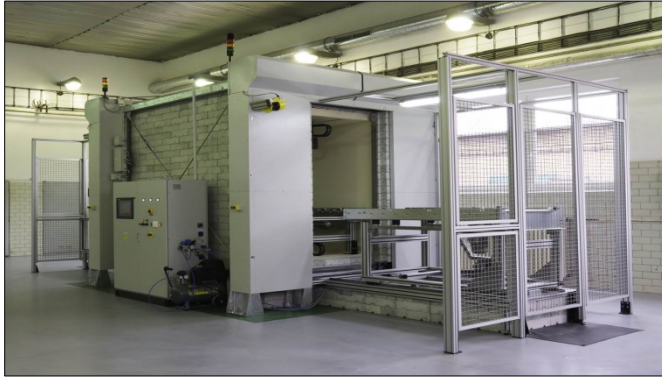
Fig. 11. Experimental Free Release Measurement System
