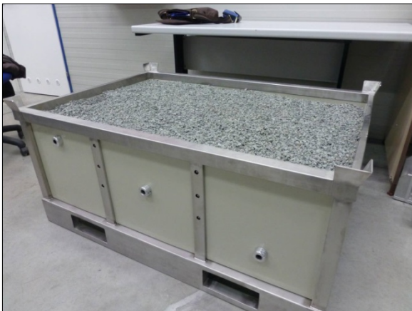
Fig. 18. Phantom filled of low radionuclide content gravel
