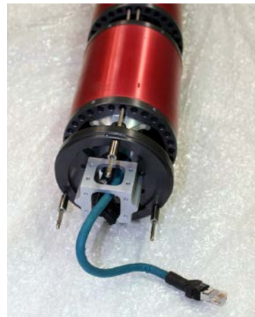
Figure 3: Mounting block attached to snake-arm robot with services
